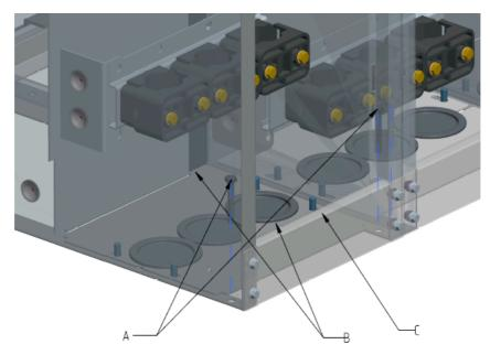
Figure 16: Positioning: Anchoring a DR-6C medium-voltage cubicle
