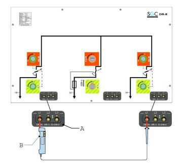
Figure 32: Measuring phase sequence
