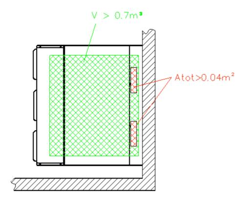
Figure 3: Top View of the installation
