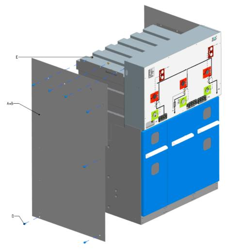
Figure 18: Assembly End Panel
