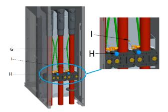
Figure 26: Assembly of the earthing cables
