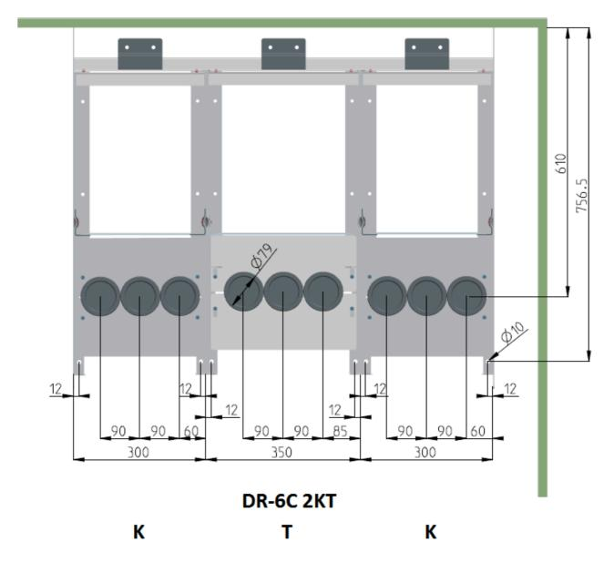
Figure 14: Positioning: Anchoring DR-6C medium-voltage switchgear
