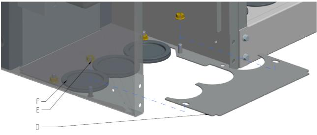
Figure 20: Disassembling the first bottom panel
