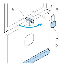
Figure 31: Placing the door back
