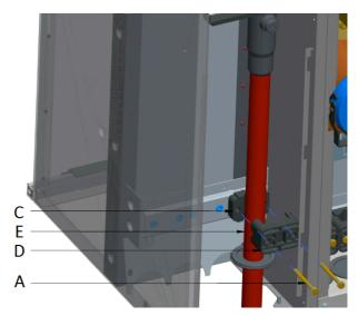
Figure 24: Assembly of the cable supports
