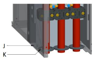
Figure 27: Positioning of the rear bottom panels
