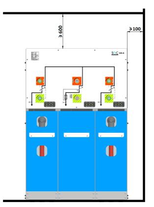
Figure 2: Minimal free height for DR-6 installation
