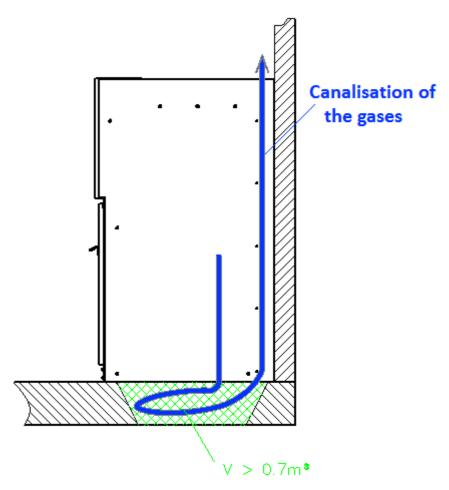
Figure 4: Diverting of the gas when installing the DR-6 RMU in a switchgear room with a cable duct (Lateral view of installation)
