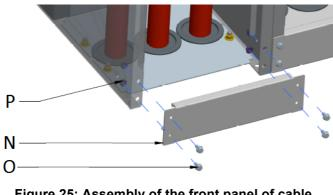
Figure 25: Assembly of the front panel of cable compartment
