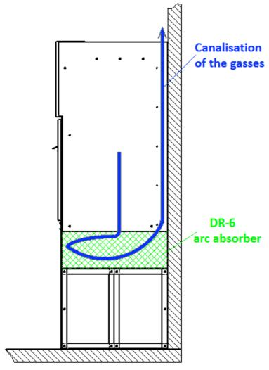
Figure 8: Diverting of the gases when installing a DR-6C arc-absorber (Lateral view of installation)
