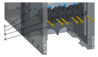
Figure 22: Assembly of the bottom panel
