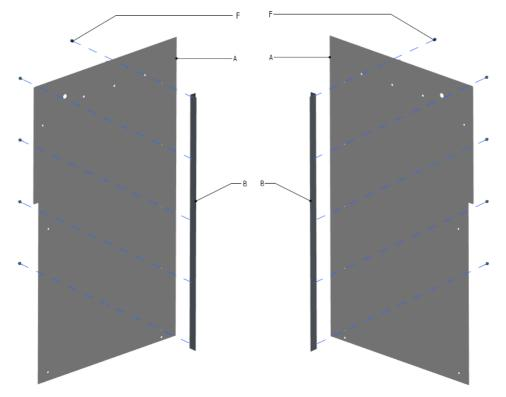
Figure 17: End panel sealing profile assembly (left and right)
