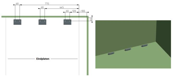
Figure 12: Positioning: Installing fixation clips
